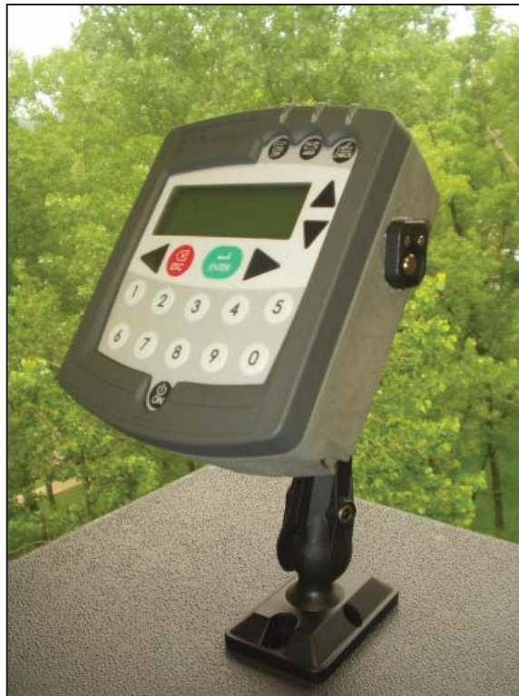
Figure 1: Example of vehicle hardware from a wireless fleet management system *
