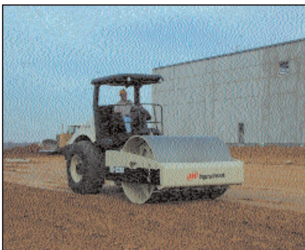
Ingersoll-Rand's new TF series SD122DX Vibratory Compactor with open ROPS replaces the Pro-Pac models. Features include drum performance, full-time traction system and improved serviceability.
