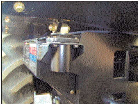
Surface Effect Platform Isolators use advanced elastomers and lubricants in a unique configuration to generate deflection-dependent damping forces.
